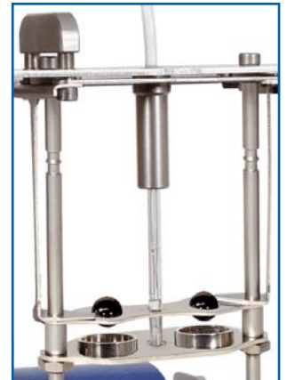
Petrotest® Ball Dispense & Centering Device (10-0840) (convenient Petrotest® setup, included in standard delivery)
