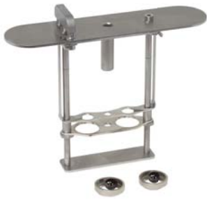
Test Rack with: mechanical Petrotest® ball centering & dispense device (10-0840 and accessories)
