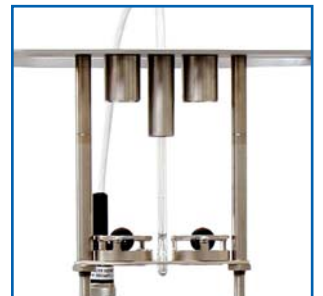
Standard Ball Centering Device (10-0841 & 2x 10-0052) (a standard setup with centering guides, substitutional for 10-0840)
